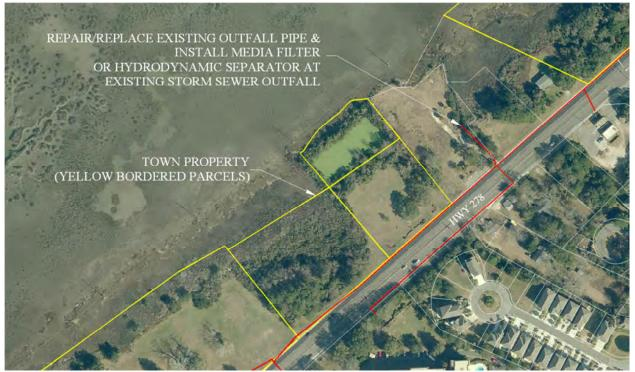
Figure 10 – Media filter/hydrodynamic separator BMP option on William Hilton Pkwy drainage outfall
