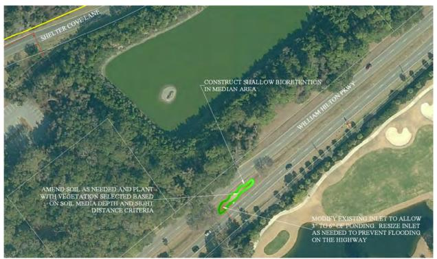
Figure 11 – Bioretention BMP option within William Hilton Pkwy median
