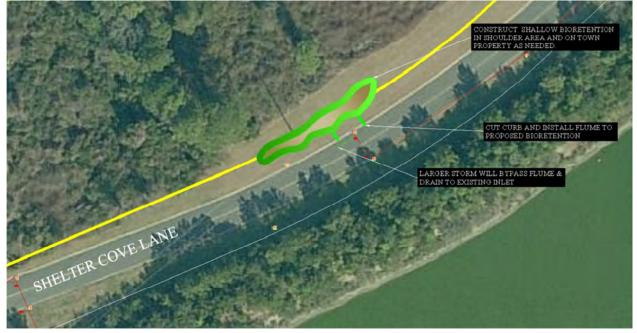
Figure 2 – Shelter Cove Lane Bioretention BMP Option
